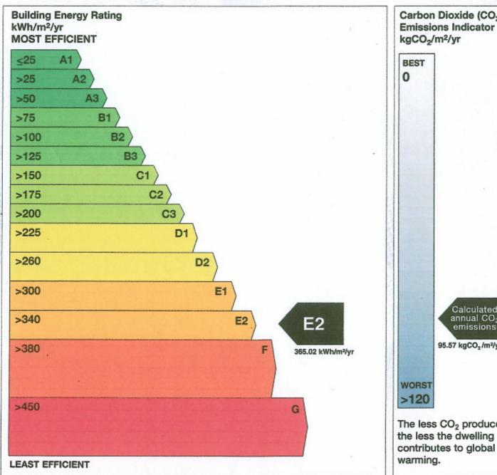
Carbon Dioxide (CO<sub>2</sub>) **Emissions Indicator** kgCO<sub>2</sub>/m<sup>2</sup>/yr Calculated annual CO<sub>2</sub> emissions 95.57 kgCO<sub>2</sub>/m<sup>2</sup>/yr WORST >120 The less CO<sub>2</sub> produced, the less the dwelling
